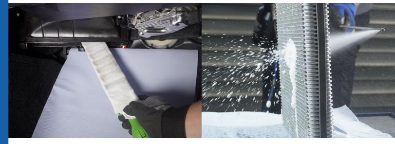
The special **airco well®** cleaner for the pollen filter box removes all dirt before inserting a new pollen filter. The housing is wiped free of residue and dirt is emoved by using the specially developed cleaning tool and a microfibre cloth soaked with cleaning chemicals. Alternatively, the cleaning aerosol can be spread in the pollen filter box using a spray probe and afterwards wiped out with a microfibre cloth.
